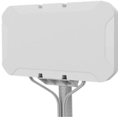
The DWMM6[X]-6-60-[X] antenna provides a 3x 2x2 MiMo omnidirectional antenna solution for global 4G/5G networks covering 617-6000MHz. It features eight separately fed ultra-wideband elements in a single housing and is suitable for a wide range of fixed-site, branch office and enterprise failover applications using cellular bonding / aggregation.
